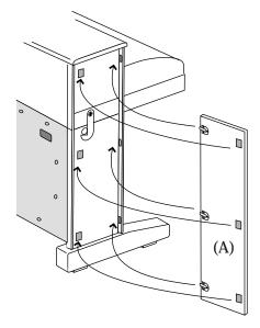
**16.** Place the Back Board (C) behind the stand and attach with ten screws (K).
